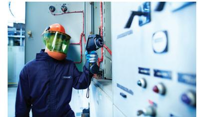
Ultrasonic testing is an excellent tool for flaw detection, such as finding compromised wiring within conduit. Using ultrasonic technology to detect and correctly identify these electrical anomalies can help prevent electrical failures and reduce life and safety risks. Ultrasonic is especially effective when used in conjunction with infrared thermography to deliver a thorough condition of maintenance assessment.
